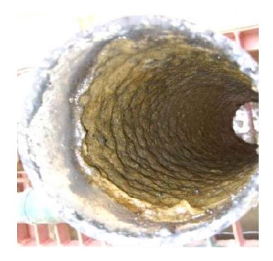
The manufacturing process requires cooling water to be delivered to the molds where the tiles are cast. The water that is used is local towns mains water and has high levels of hardness. Part of the problem was the low flow rate in the pipe line due to heavily scale pipe.
