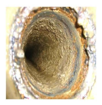
Once the MagCat was removed it was clear that the MagCat was having a considerable effect on the system. The scale thickness had decreased from 10mm to 3mm, a drop of 7mm.
