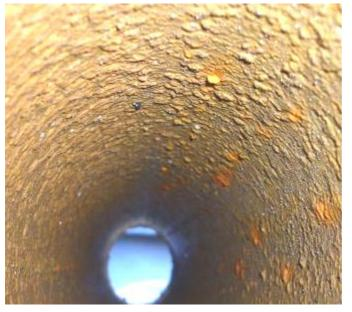
Before: 26-12-09 Picture of scale inside pipe before installed CAT-100 Thickness 2.00 - 3.00 mm..
