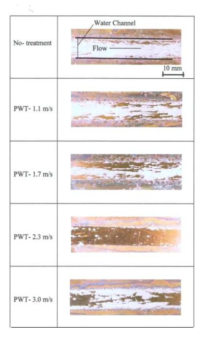
Fig.3 Photographs of fouled surfaces taken after the fouled heat-Transfer surfaces were completely dried
