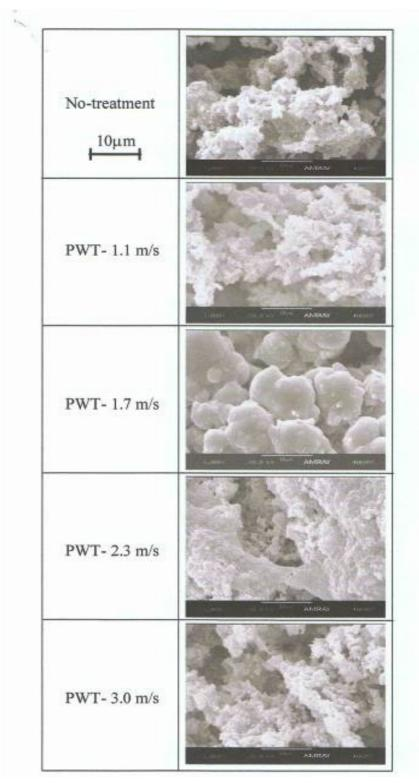
Fig. 4 SEM photographs for all cases , 3000X Velocity Effect with PWT - 17
