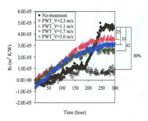
Fig.1 Variations of fouling resistance vs. time for four different flow velocity cases through PWT
