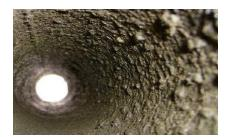
Feed Line to compressors with scale deposition
