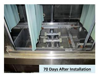
The Challenge: Even though properly maintained a conventional salt based water softener at Fort Bend ISD (Independent School District) had proven to be ineffective at preventing scale. This resulted in scaling throughout the system particularly in the kitchen / cafeteria area. The main Hobart dishwashing equipment had to be opened up and descaled every week taking up staff time and consuming chemicals. Trays and dinnerware showed noticeable signs of scale.
