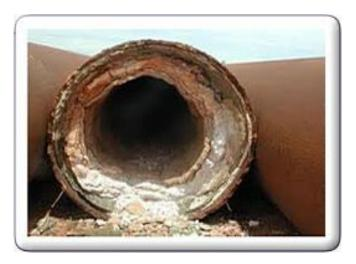
One area where scale will cause a problem is deposition inside the main feed pipes. Particularly hard water will see a steady build up of scale inside the pipe. This causes a reduction in water delivery, increasing the workload on the pumps. Furthermore scale can also contribute to corrosion of the pipe itself.
