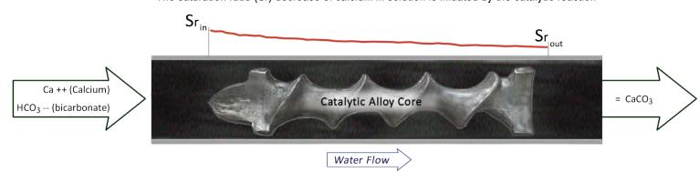
When calcium precipitates in this way it can combine with bicarbonate to form a hard calcium carbonate scale called calcite that bonds to the nearest receptive surface.
