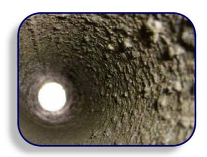
Scale formation inside compressors is caused by the deposition of calcium carbonate from hard water that is used to cool the compressor.
