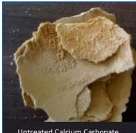
Untreated Calcium Carbonate formed as hard scale
