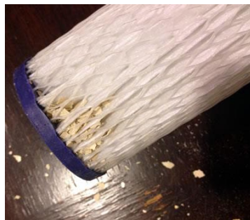
Scale in Washing Machine Filter
